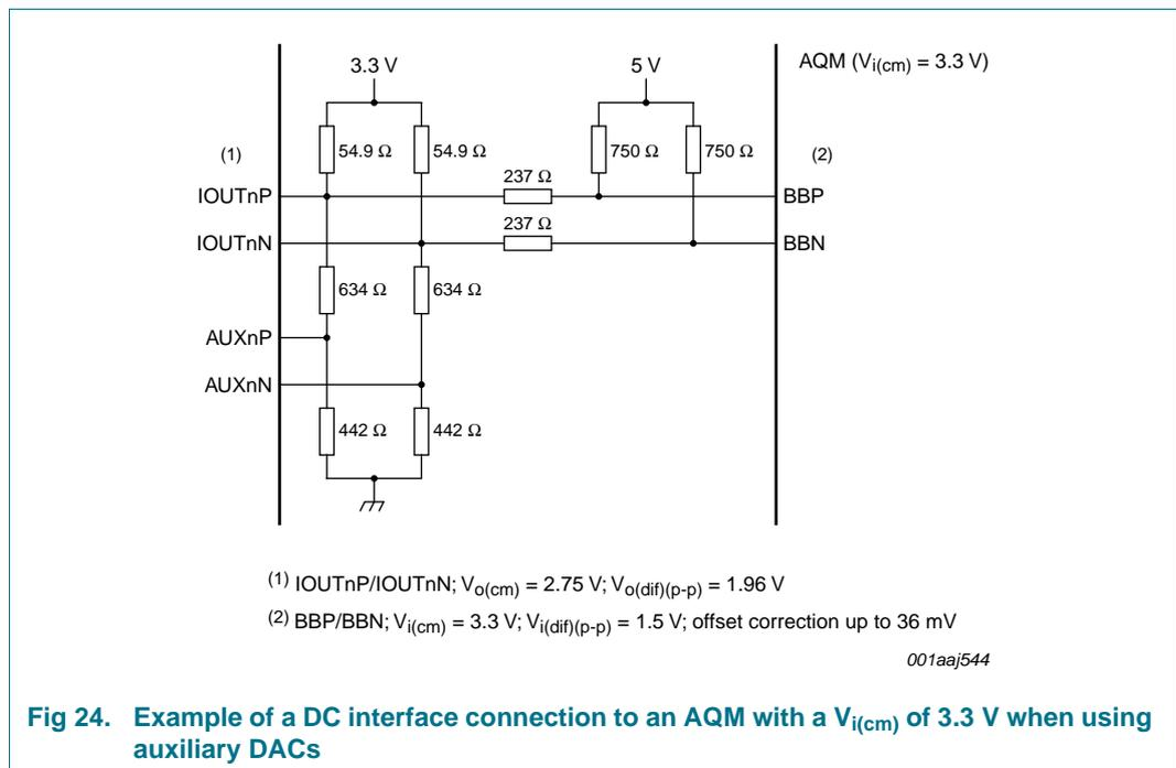
The constraints to adjusting the interface are the output compliance range of the DAC and the auxiliary DACs, the input common-mode level of the AQM, and the range of offset correction.
