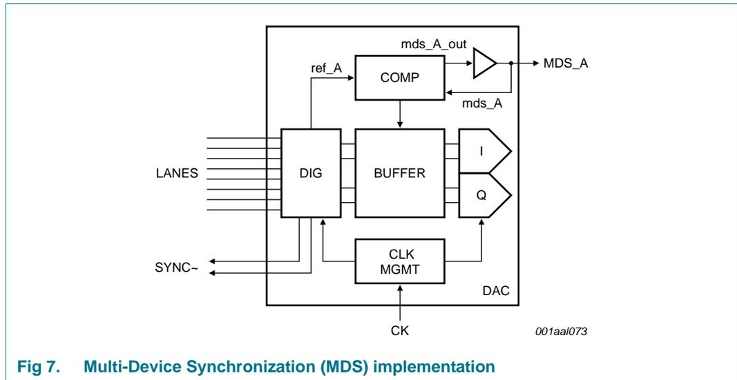
**Fig 7. Multi-Device Synchronization (MDS) implementation**
