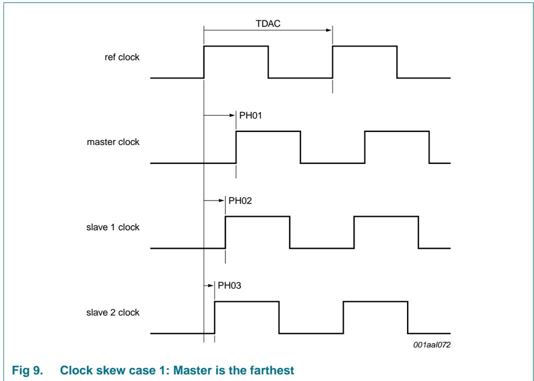
**Fig 9. Clock skew case 1: Master is the farthest**
