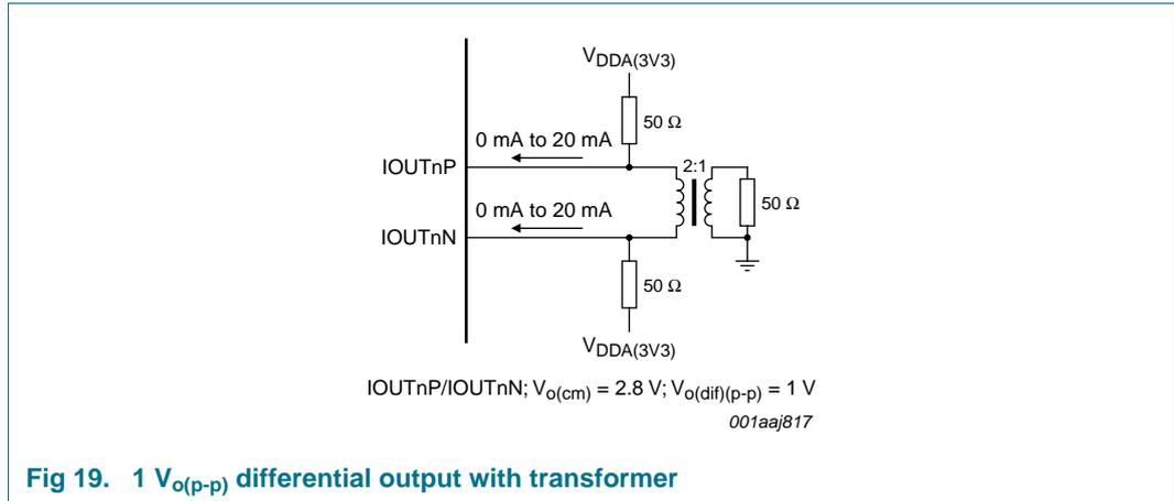
**Fig 19. 1 V<sub>o(p-p)</sub> differential output with transformer**
