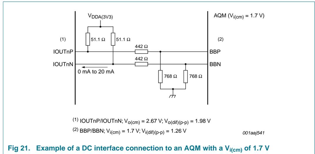
Fig 21. Example of a DC interface connection to an AQM with a  $V_{i(cm)}$  of 1.7 V
