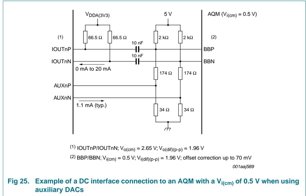
Fig 25. Example of a DC interface connection to an AQM with a  $V_{i(cm)}$  of 0.5 V when using auxiliary DACs
