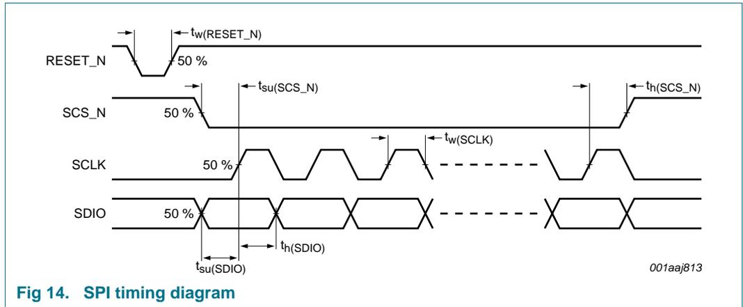
Fig 14. SPI timing diagram
