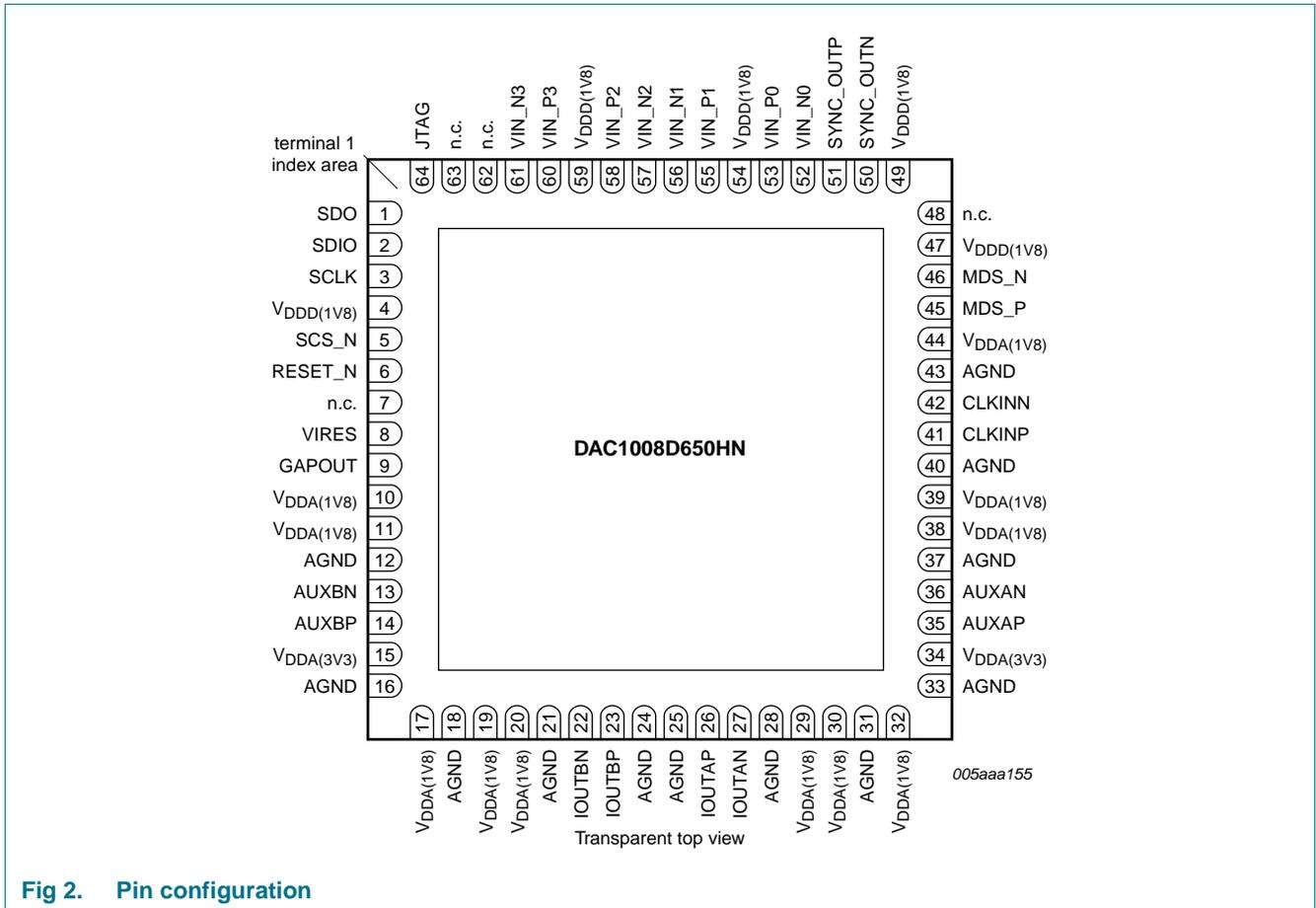
Fig 2. Pin configuration
