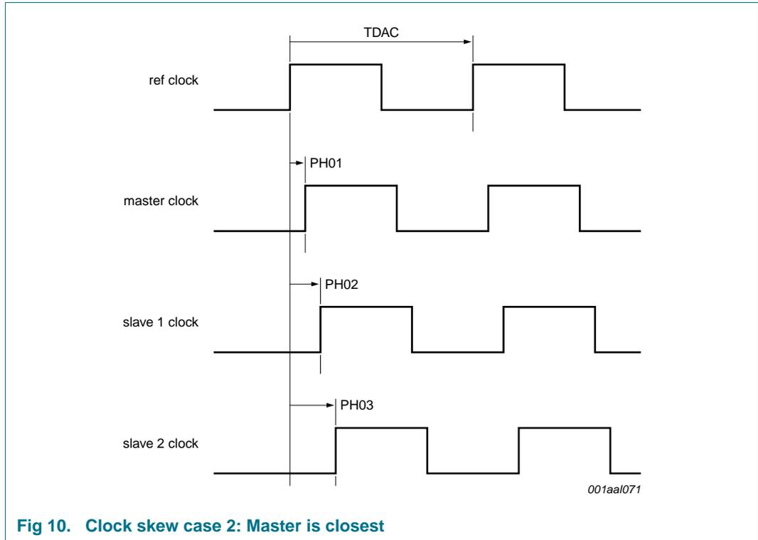
**Fig 10. Clock skew case 2: Master is closest**
