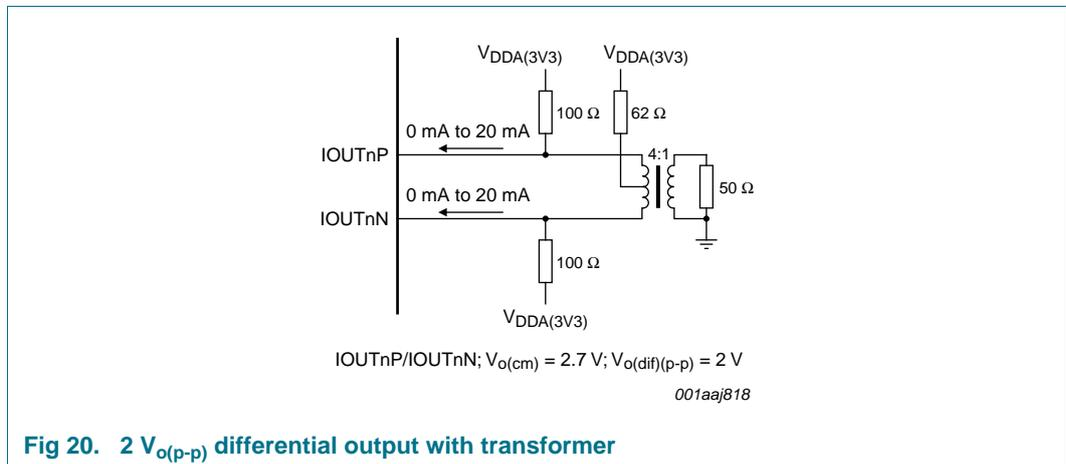
**Fig 20. 2 V<sub>o(p-p)</sub> differential output with transformer**
