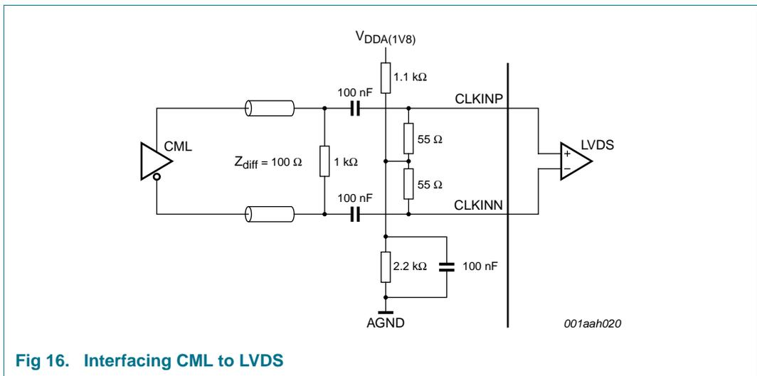
Fig 16. Interfacing CML to LVDS
