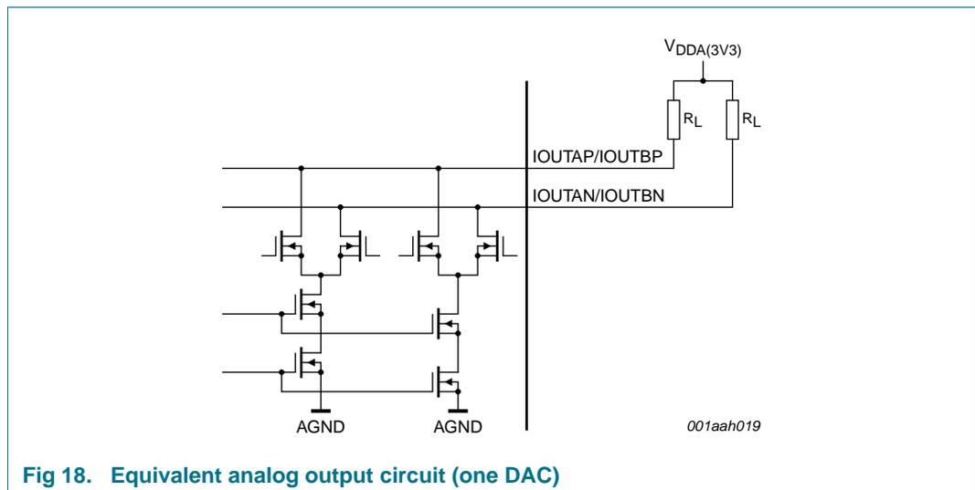
**Fig 18. Equivalent analog output circuit (one DAC)**
