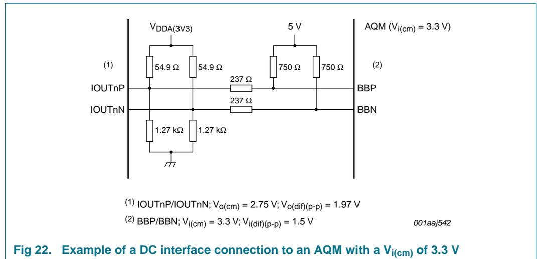
Fig 22. Example of a DC interface connection to an AQM with a  $V_{i(cm)}$  of 3.3 V
