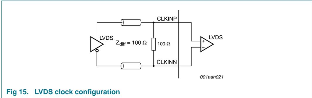
Fig 15. LVDS clock configuration
