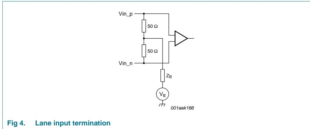
**Fig 4. Lane input termination**
