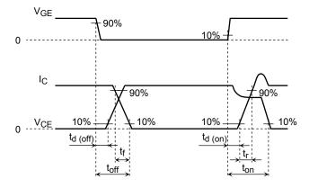
Note 2: Switching loss measurement waveforms
