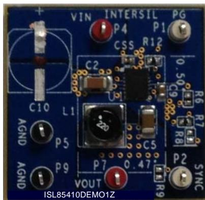
FIGURE 1. FRONT OF EVALUATION BOARD ISL85410DEMO1Z
