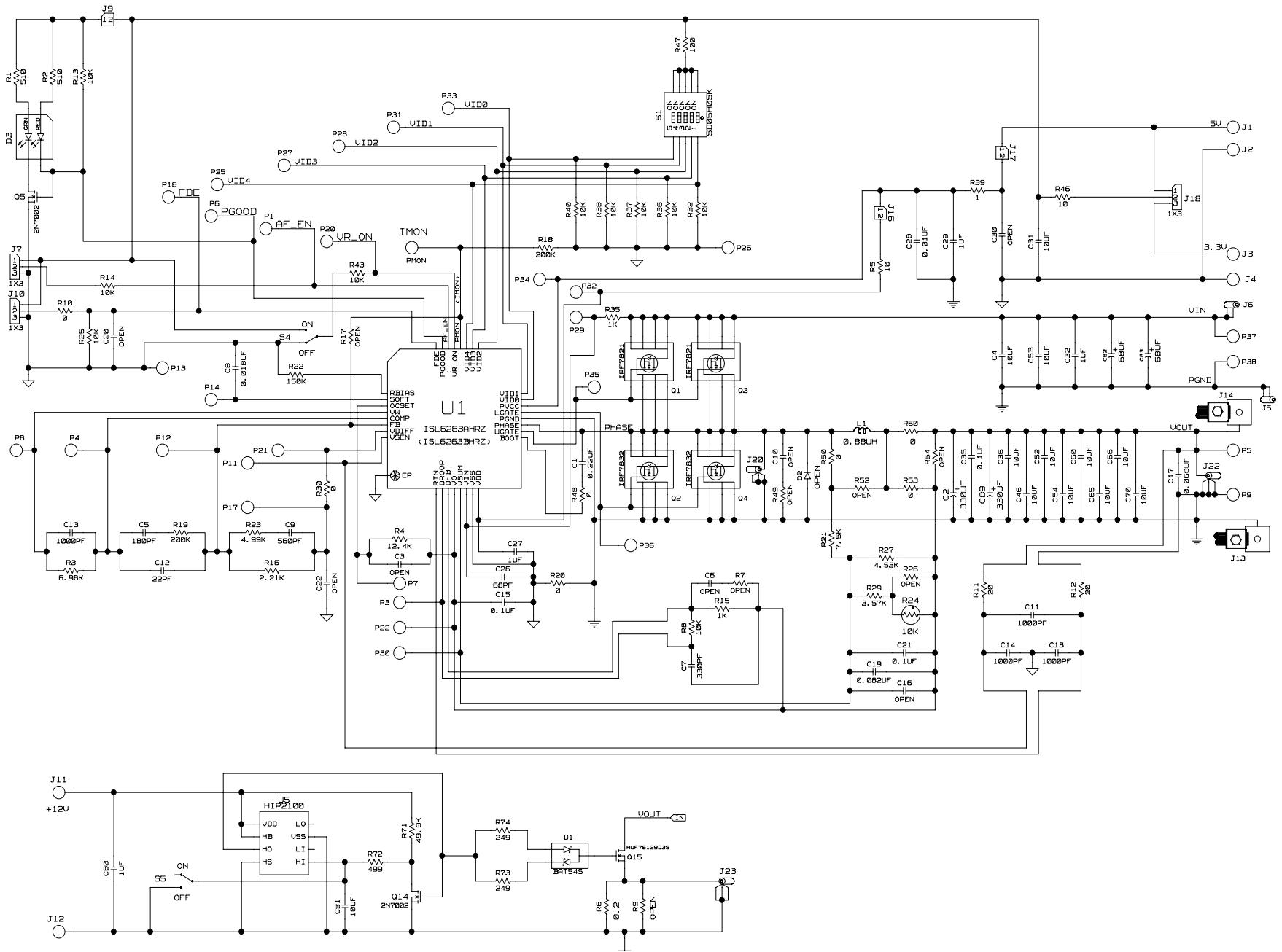
**FIGURE 1. ISL6263AEVAL1Z AND ISL6263BEVAL1Z EVALUATION BOARDS SCHEMATIC**
