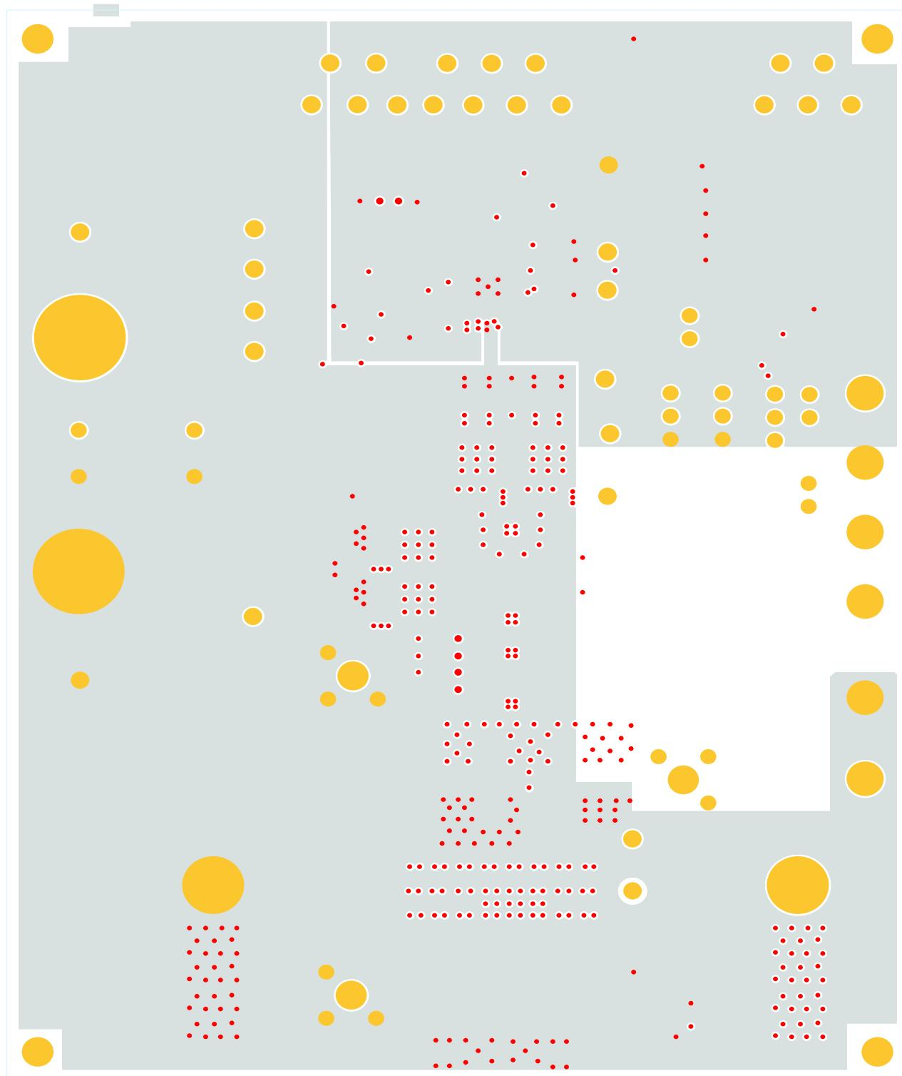
FIGURE 5. ISL6263AEVAL1Z and ISL6263BEVAL1Z EVALUATION BOARDS LAYER 2 ETCH
