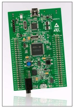
Based on the STM32F407VGT6, it includes an ST-LINK/V2 embedded debug tool, two ST MEMS, digital accelerometer and digital microphone, one audio DAC with integrated class D speaker driver, LEDs and push buttons and an USB OTG micro-AB connector.
