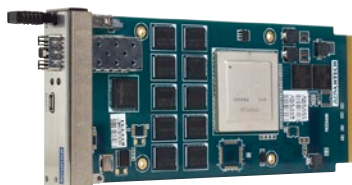
Figure 2: Advantech AMC-4201 AdvancedMC™ board featuring the QorIQ P4080 processor
