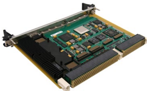
Figure 3: Curtiss Wright VPX6-187 based on the QorIQ P4080 processor
