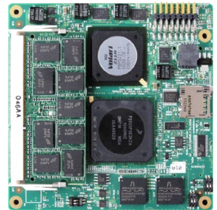
Figure 1: Emerson Network Power COM Express™ compatible module based on the QorIQ P2020 processor
