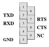
Female DB9 connector that interfaces to the HCS08 internal SCI1 serial port via the U2 RS232 transceiver. It provides simple 2 wire asynchronous serial communications without flow control. Flow control is provided at test points on the module.
