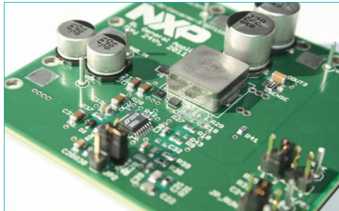
Demo-PCB DC-DC down-conversion with 2 PMPBEN MOSFETs Condition: V_{in} = 10\text{ V} ; V_{out} = 1.5\text{ V @ } 6\text{ A} ; f_{sw} = 490\text{ kHz}
