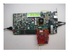
Start IMPACT, and initialze the JTAG chain. The program should recognize the 7 series device. Start a UART terminal (set to 57600 baud rate) and then program the device. If programming was successful, you should be seeing messages appear on the terminal as shown in figure below. After programming the devices, the program checks data capture on various test modes.
