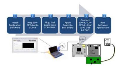
For successful SDP-FPGA and Evaluation board installation, follow these steps:
