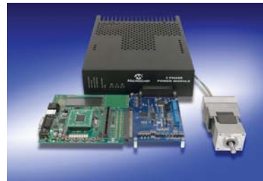
A 3-phase Low Voltage Power Module with Explorer 16 Board, Motor Control Interface Board and a Hurst Motor are shown.
