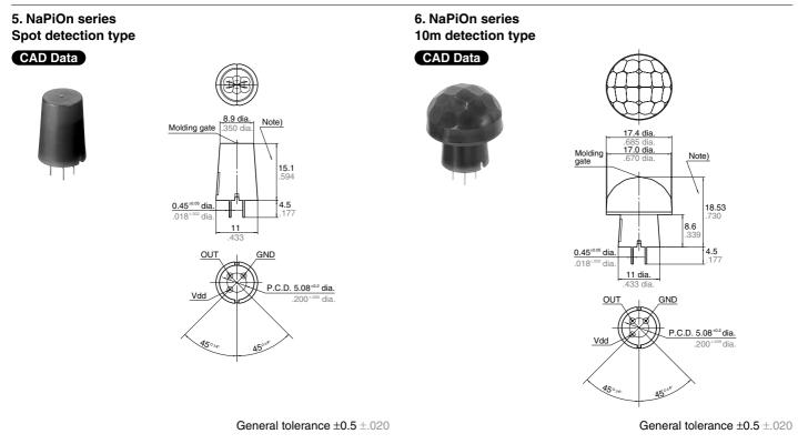
Note: The height dimension does not include the remaining molding gate.
