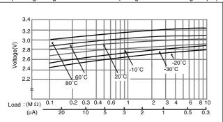
■ Capacity vs. load resistance
