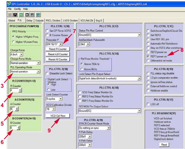
Figure 13. PLL Configuration for the 122.88 MHz Crystal Oscillator
