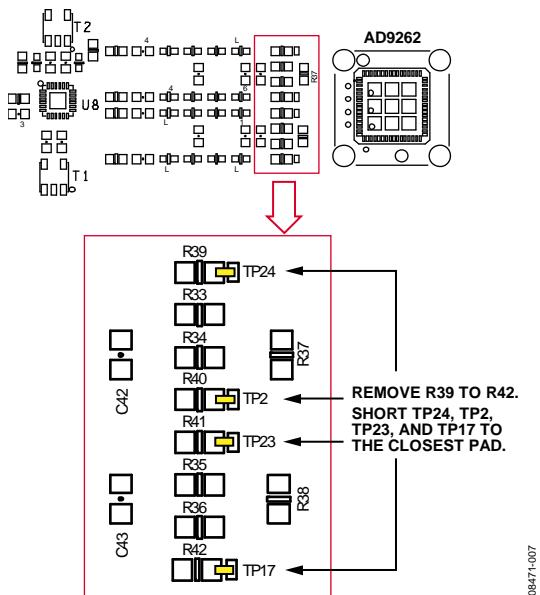
*Figure 7. External ADC Jumper Settings***DIFFERENTIAL TRANSFORMER PATH**
