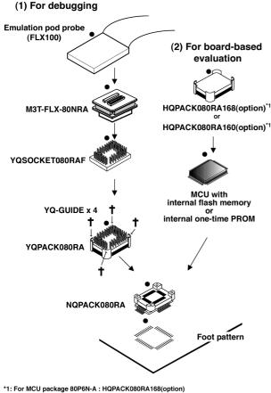
\*1: For MCU package 80P6N-A : HQPACK080RA168(option) For MCU package 80P6U-A : HQPACK080RA160(option)
