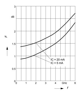
Noise figure  $F = f(I_C)$  $V_{CF} = 2 V, f = 1.8 \text{ GHz}$
