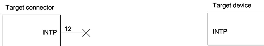
**Figure 5-9. Circuit Connection for the Case Where MINICUBE2 Is Used for Debugging and Debugging of INTP Pin Is Performed Only with Real Machine**
