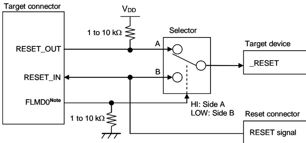
**Note** FLMD0 is high level when MINICUBE2 is connected, and FLMD0 is pulled down when MINICUBE2 is not connected.
