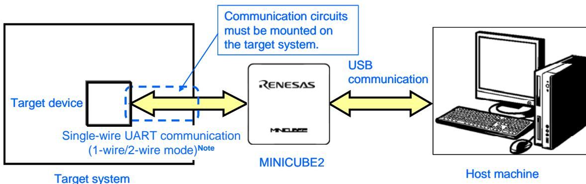
**Note** 1-wire mode: Single-wire UART communication using TOOL0 pin
