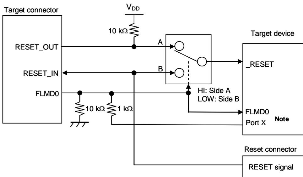
**Note** This circuit is designed for flash self programming, which controls the FLMD0 pin via ports.
