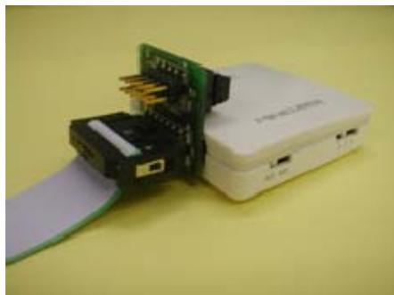
**Caution** Connect the 78K0-OCD board to the target cable so that pin 1 position (▲) on each side match.
