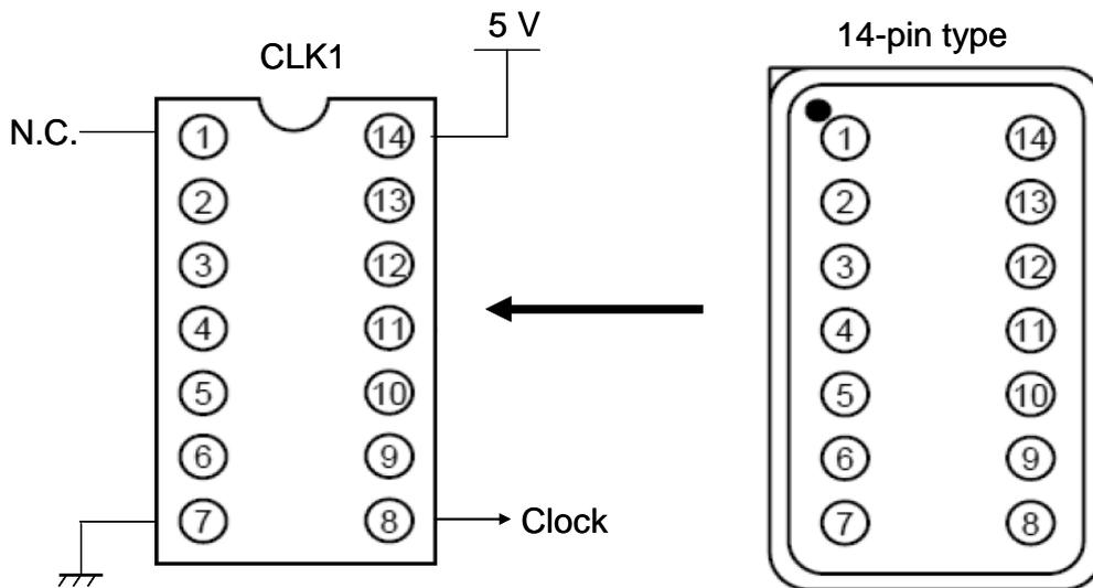
**(d) Using the oscillator circuit connected to the 78K0-OCD board (only when OCD0A and OCD0B or TOOLD0 and TOOLC0 are used)**
