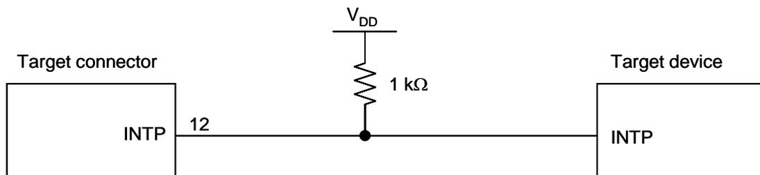
**Figure 5-8. Circuit Connection for the Case Where MINICUBE2 Is Used Only for Programming**
