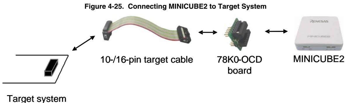
**<R> Caution** On-chip debugging using TOOLCx and TOOLDx can be performed without using the 78K0-OCD board. When TOOLC0 and TOOLD0 are used, a 4, 8, or 16 MHz clock signal generated by MINICUBE2 can be used for the clock signal of the microcontroller.
