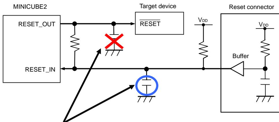
If a capacitance element such as a capacitor or resistor is connected to the RESET\_OUT pin, the target device might not be able to communicate with MINICUBE2.
