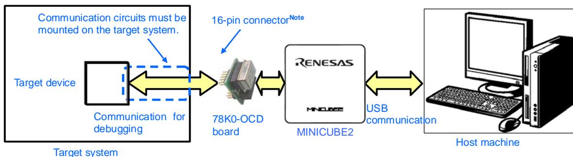
**Note** To reduce the footprint of the target system, SICA can be used to reduce the size of connectors. When replacing QB-78K0MINI (obsolete product) with MINICUBE2, a 10-pin connector dedicated to debugging can be used.
