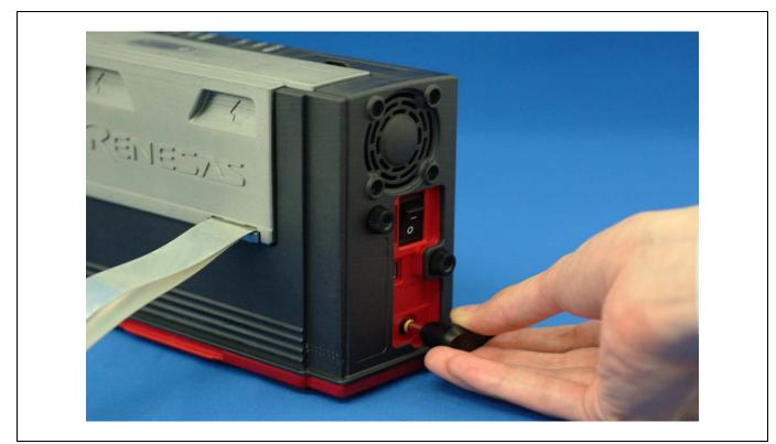
Figure 2.5 Connecting the emulator power supply
