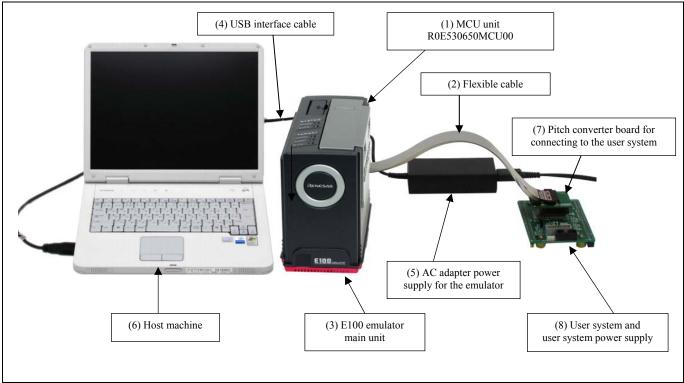
Figure 1.1 System configuration
