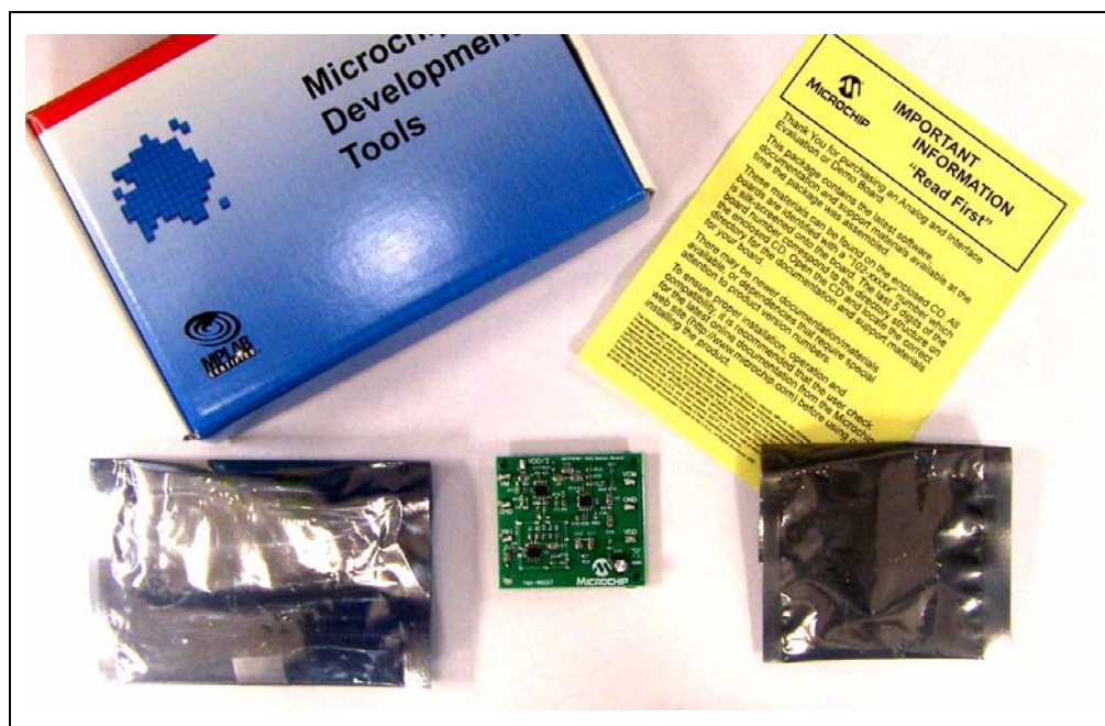
FIGURE 1-1: MCP6V01 Input Offset Demo Board Contents.
