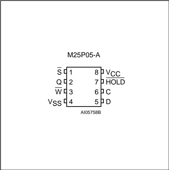
Figure 3. SO, VDFPN and TSSOP Connections
