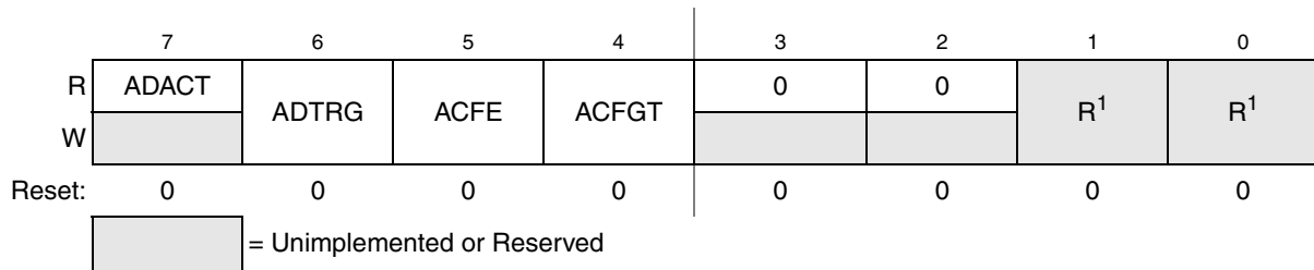
Figure 9-5. Status and Control Register 2 (ADCSC2)
