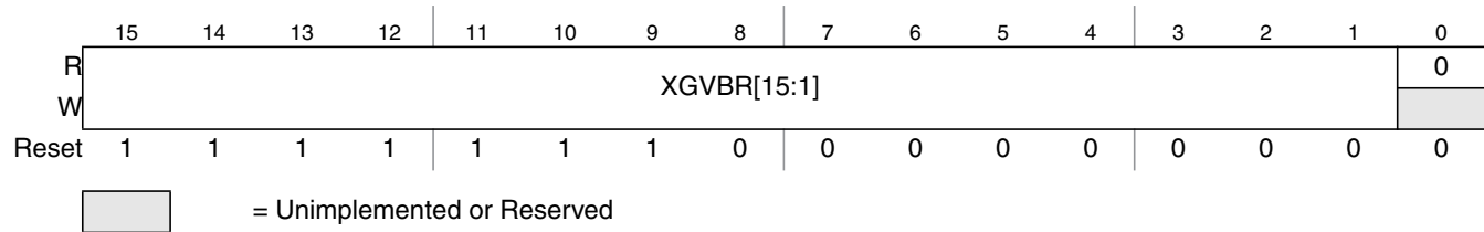
Figure 10-9. XGATE Vector Base Address Register (XGVBR)
