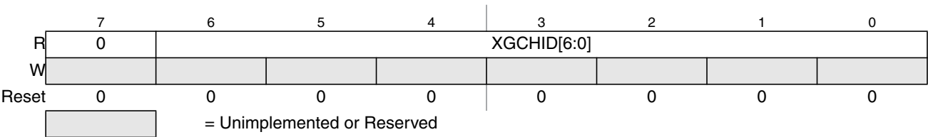
Figure 10-4. XGATE Channel ID Register (XGCHID)
