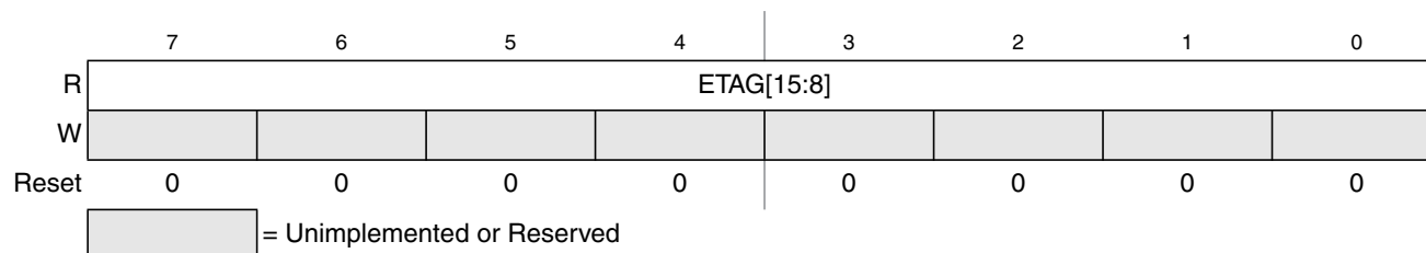
Figure 27-18. EEE Tag Counter High Register (ETAGHI)
