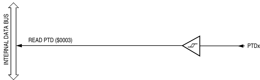
Figure 10-12. Port D Input Circuit
