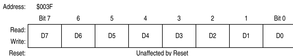
Figure 27-20. BDLC Data Register (BDR)
