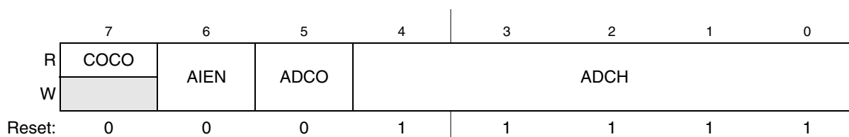
Figure 10-3. Status and Control Register (ADCSC1)
