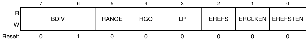
Figure 12-4. MCG Control Register 2 (MCGC2)
