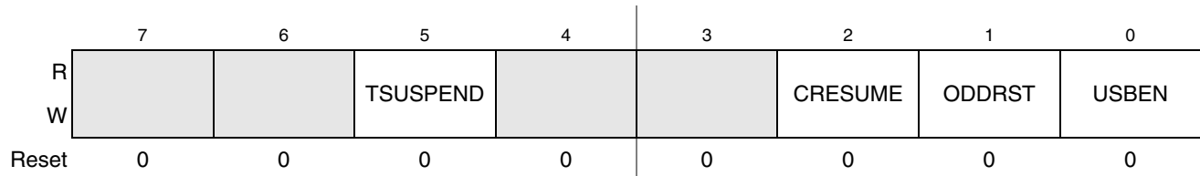
Figure 17-13. Control Register (CTL)
