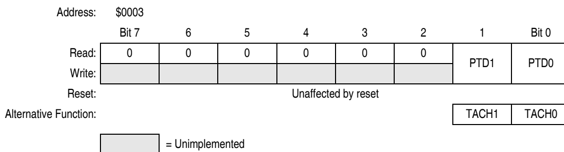
Figure 12-10. Port D Data Register (PTD)
