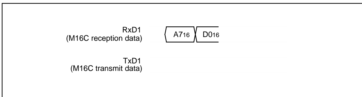
Figure 32.26 Timing for erasing all unlocked blocks
