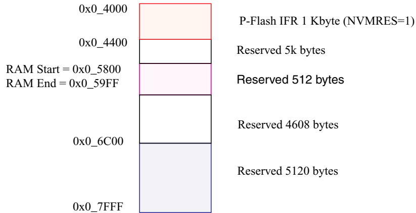
Figure 17-2. Memory Controller Resource Memory Map (NVMRES=1)
