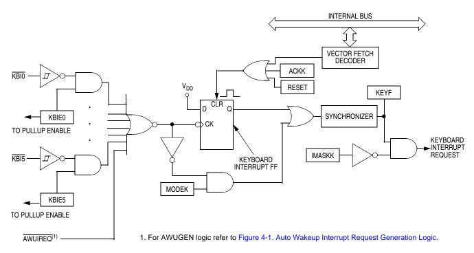
Figure 9-2. Keyboard Interrupt Block Diagram
