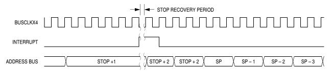
Figure 13-18. Stop Mode Recovery from Interrupt
