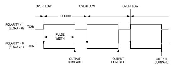
Figure 14-3. PWM Period and Pulse Width
