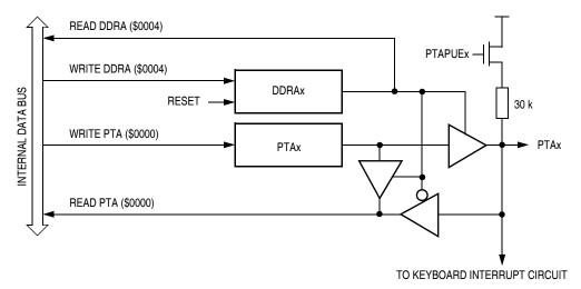
Figure 12-3. Port A I/O Circuit
