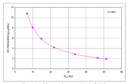
Figure 16-8. RC versus Frequency (3 Volts @ 25•C)
