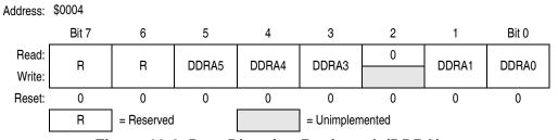
Figure 12-2. Data Direction Register A (DDRA)
