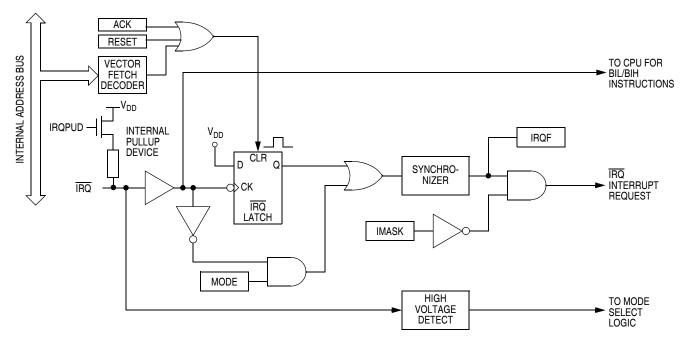
Figure 8-2. IRQ Module Block Diagram
