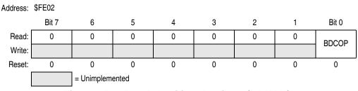
Figure 15-6. Break Auxiliary Register (BRKAR)
