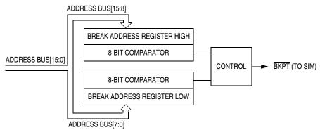
Figure 15-2. Break Module Block Diagram
