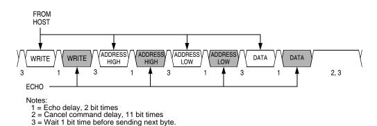
Figure 15-16. Write Transaction
