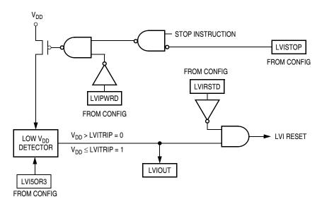
Figure 10-1. LVI Module Block Diagram
