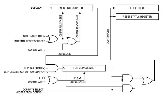
Figure 6-1. COP Block Diagram
