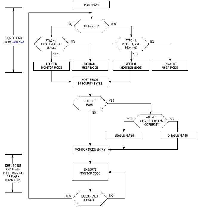
Figure 15-9. Simplified Monitor Mode Entry Flowchart
