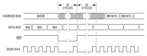
Figure 13-16. Wait Recovery from Internal Reset
