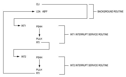
Figure 13-10. Interrupt Recognition Example
