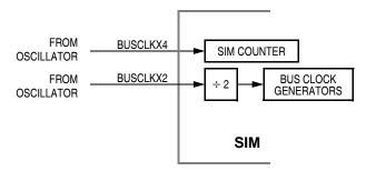
Figure 13-2. SIM Clock Signals
