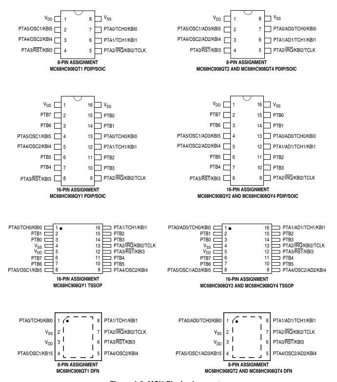
Figure 1-2. MCU Pin Assignments
