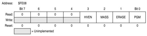
Figure 2-3. FLASH Control Register (FLCR)
