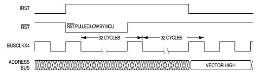
Figure 13-4. Internal Reset Timing
