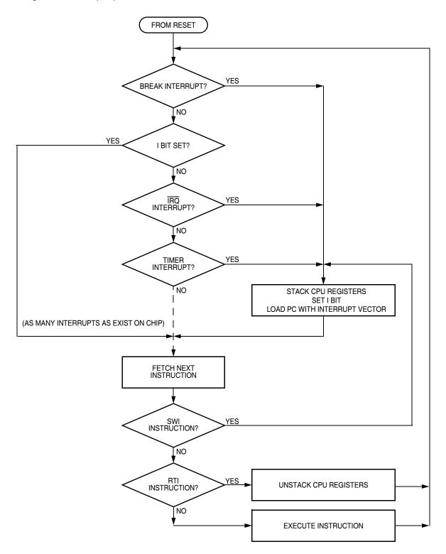
Figure 13-7. Interrupt Processing
