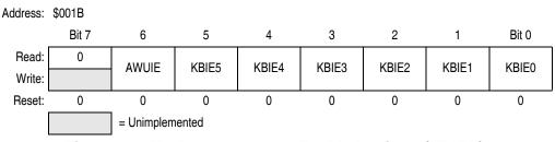
Figure 9-4. Keyboard Interrupt Enable Register (KBIER)
