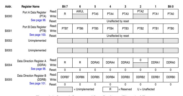
Figure 2-2. Control, Status, and Data Registers (Sheet 1 of 5)
