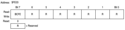
Figure 13-20. Break Flag Control Register (BFCR)
