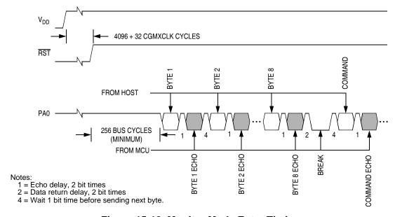
Figure 15-18. Monitor Mode Entry Timing
