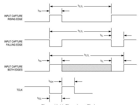
Figure 16-11. Timer Input Timing
