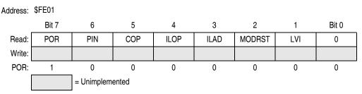
Figure 13-19. SIM Reset Status Register (SRSR)
