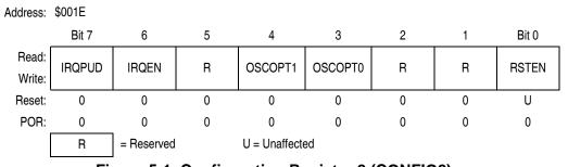
Figure 5-1. Configuration Register 2 (CONFIG2)
