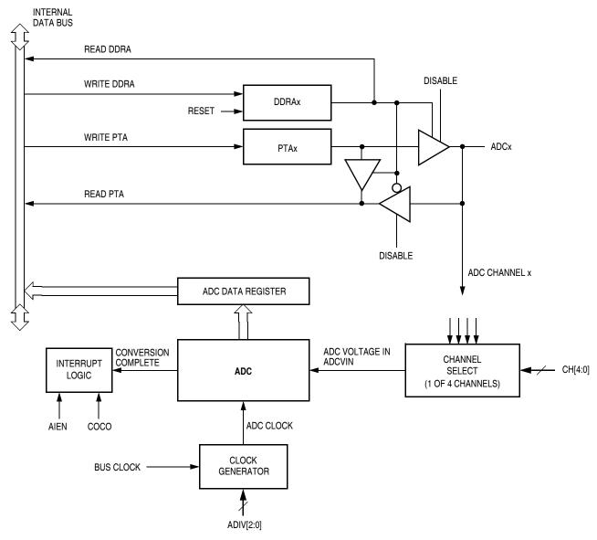
Figure 3-2. ADC Block Diagram
