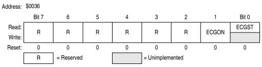
Figure 11-4. Oscillator Status Register (OSCSTAT)
