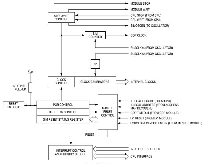
Figure 13-1. SIM Block Diagram
