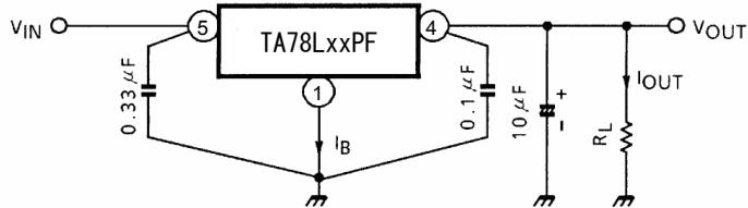
Use capacitors to connect the input terminal and GND and the output terminal and GND. The capacitances should be determined experimentally. In particular, adequate investigation should be made to ensure there is no problem even in high or low temperatures.
