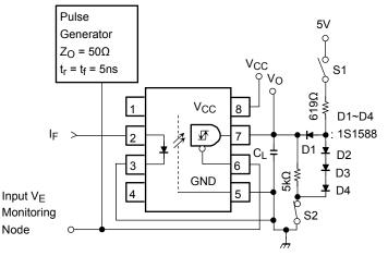
$\ensuremath{\mathsf{C}}\xspace_{\mathsf{L}}$  is approximately 15pF which includes probe and stray wiring capacitance.
