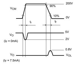
$$\text{CM}_H = \frac{160(\text{V})}{t_\text{f}(\mu \text{s})}, \text{CM}_L = \frac{160(\text{V})}{t_\text{f}(\mu \text{s})}$$
