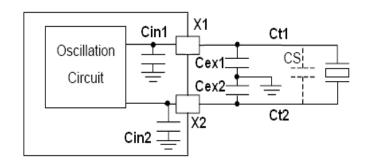
In the above figure, X1 and X2 are the crystal pins of our device. Cin1 and Cin2 are the internal capacitors which include the X1 and X2 pin capacitance. Cex1 and Cex2 are the external capacitors that are needed to tune the crystal frequency. Ct1 and Ct2 are the PCB trace capacitances between the crystal and the device pins. CS is the shunt capacitance of the crystal (as specified in the crystal manufacturer's datasheet or measured using a network analyzer).
