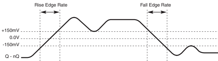
DIFFERENTIAL MEASUREMENT POINTS FOR RISE/FALL TIME
