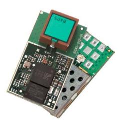
The BTM520 and BTM521 are the most advanced low-power multimedia Bluetooth® modules available in the marketplace. Designed to meet the needs of developers requiring ultimate Bluetooth audio performance and flexibility, these modules include everything required for a fully qualified and functional Bluetooth multimedia application.
