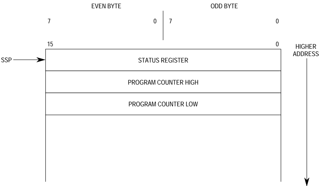
Figure 2-4. M68000 Short-Form Exception Stack Frame
