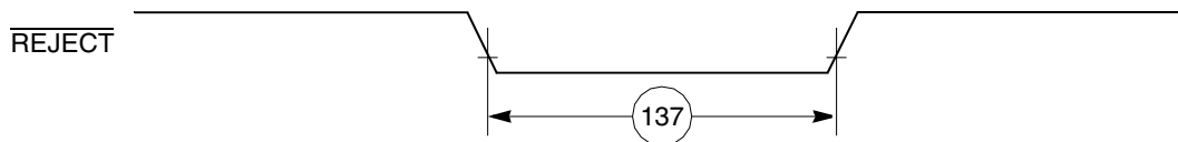
Figure 63. CAM Interface \overline{\text{REJECT}} Timing Diagram
