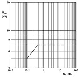
Maximum allowed peak pulse voltage in accordance with IEC 60065, 14.1.a; 50 discharges from a 1 nF capacitor charged to  $\hat{U}_{max}$ .; 12 discharges/min (drift  $\Delta R/R \le 2$  %)
