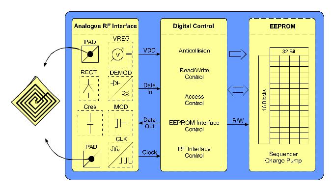
The label requires no internal power supply. Its contactless interface generates the power supply and the system clock via the resonant circuitry by inductive coupling to the reader. The interface also demodulates data that are transmitted from the reader to the I•CODE Label, and modulates the electromagnetic field for data transmission from the I•CODE Label to the reader.
