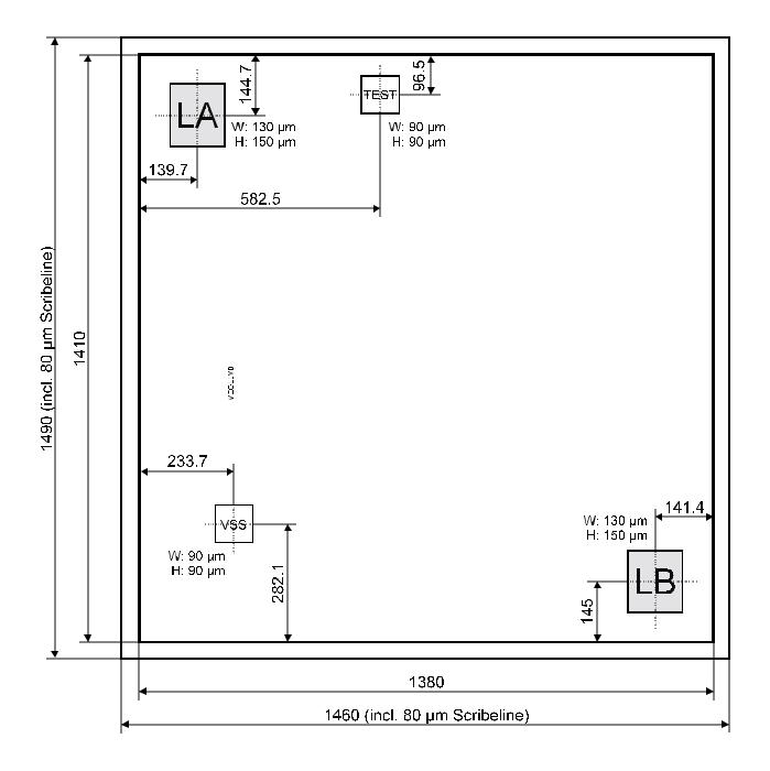
Measuring unit: µm
