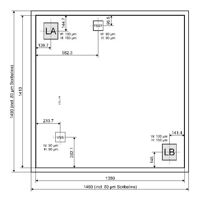
Measuring unit: µm
