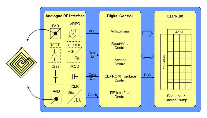
The label requires no internal power supply. Its contactless interface generates the power supply and the system clock via the resonant circuitry by inductive coupling to the reader. The interface also demodulates data that is transmitted from the reader to the I•CODE Label and modulates the electromagnetic field for data transmission from the I•CODE Label to the reader.
