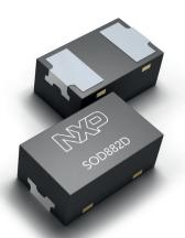
NXP SOD882D package with reduced height and innovative pad design
