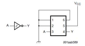
$<sup>^{\</sup>star}$  Note: Since the B and C inputs are hard-wired to GND, toggling the B and C switches does not impact gate function.
