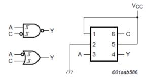
$<sup>^{\</sup>star}$  Note: since the B input is hard-wired to Vcc, toggling the B switch does not impact gate function.
