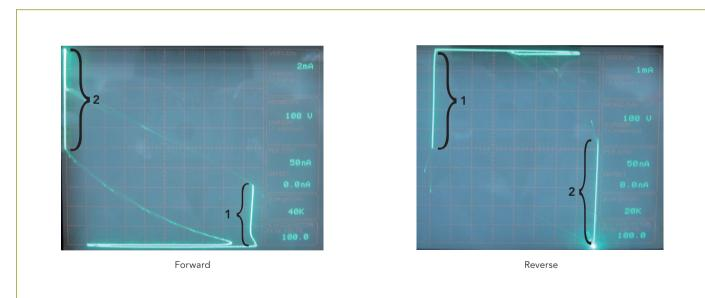
1 - During low-energy overvoltage transients, safe clamping minimizes false triggers caused by inductive load back-EMF at commutation 2 - During high-energy overvoltage transients, the ACT automatically turns on, thus letting energy dissipate safely in the load
