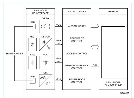
Fig 1. Block diagram of HITAG 1 transponder IC
