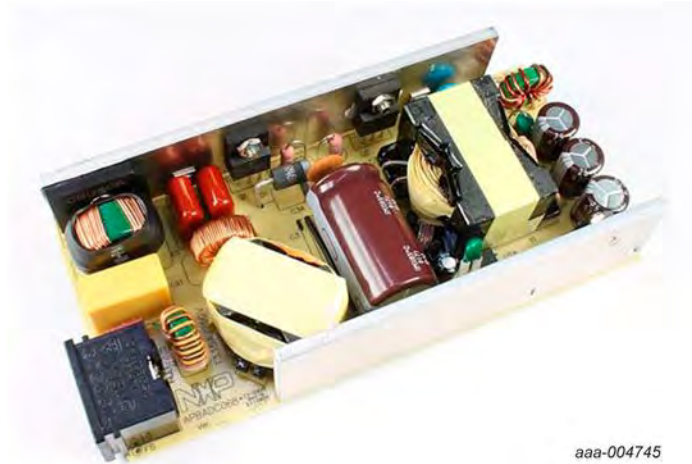
Fig 1. 90 W TEA1755T, TEA1792TS and TEA1703TS demo board (top view)
