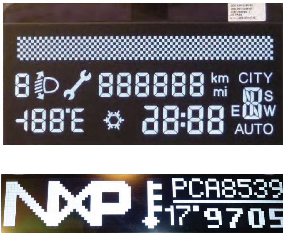
Fig 5. Displays of the demo boards driven by the PCA8538 and PCA8539
