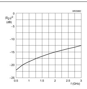
Diode zero biased and inserted in series with a 50  $\Omega$  stripline circuit.  $T_{amb}$  = 25 °C.
