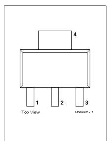
Fig.1 Simplified outline (SOT223) and pin configuration.
