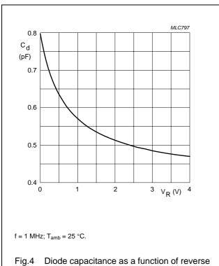
Ig.4 Diode capacitance as a function of reve voltage; typical values.
